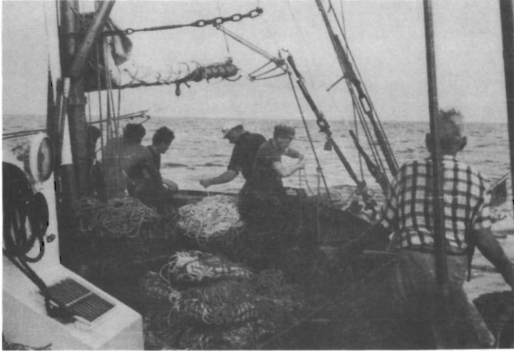
Photo 1. Shooting the longline. The baskets of longline in the foreground are still in their net wrappers, while an unwrapped basket in the background is being shot over the side.
