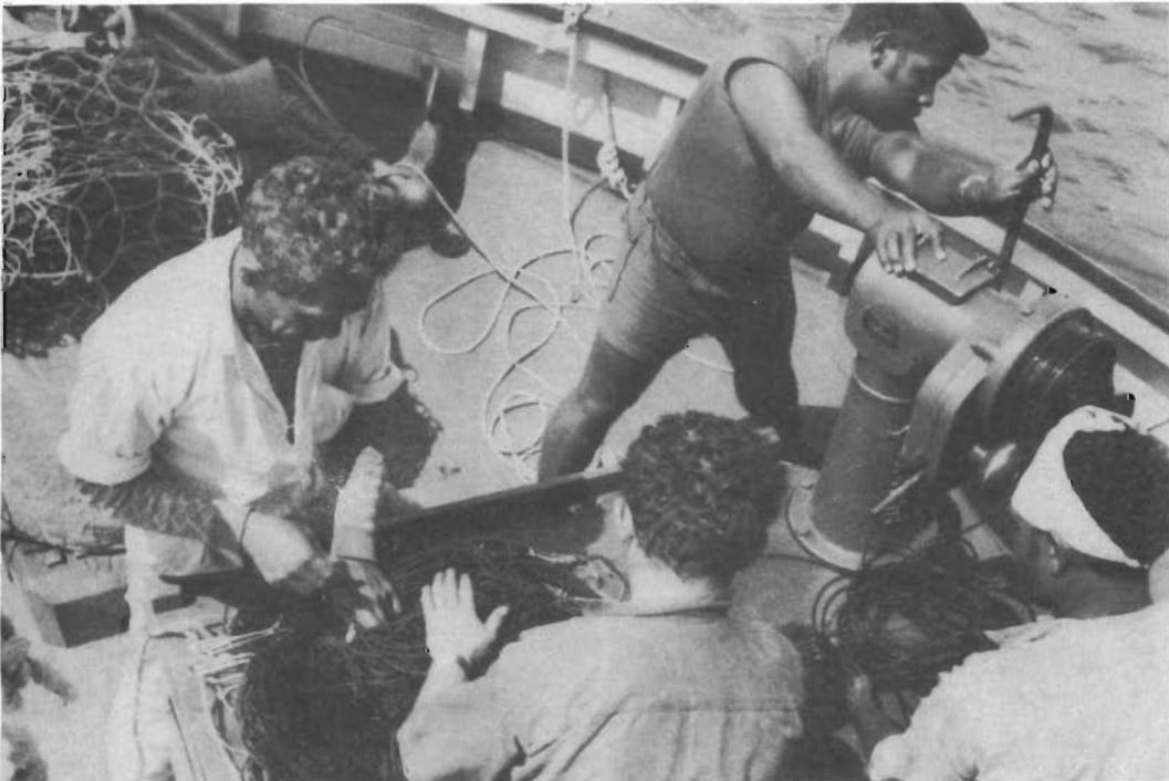
Photo 2. Hauling in the line. Visible at lower left, the snap fasteners of the main line, snapped in their respective order on one side of the net wrapper.
