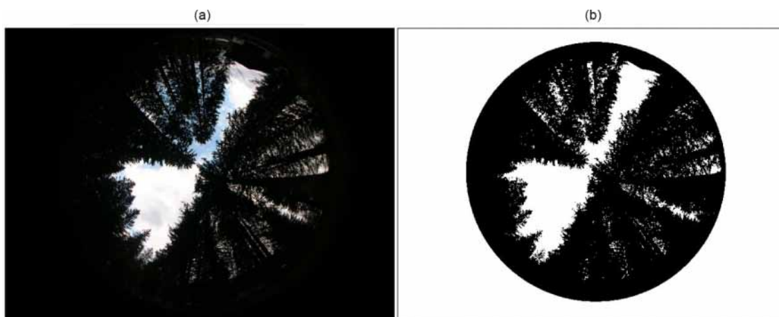
Figure 5. Example of a hemispherical photograph (a) and a binary image (b); white pixels are sky and black pixels are canopy, calculated with a sky view factor of 0.25). The photograph was taken on 4 September 2017 at radiometer A1 (Fig. 1).
