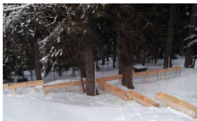
Figure 7. Precipitation tanks installed below the canopy (photograph by Yves Lejeune).
