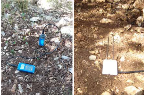
Fig. 17. Photos of soil moisture measurements at PSL on plot 22 (left, photo by Karine Adeline, ONERA) and at PUE (right, photo by Jean-Marc Limousin, CEFÉ).
