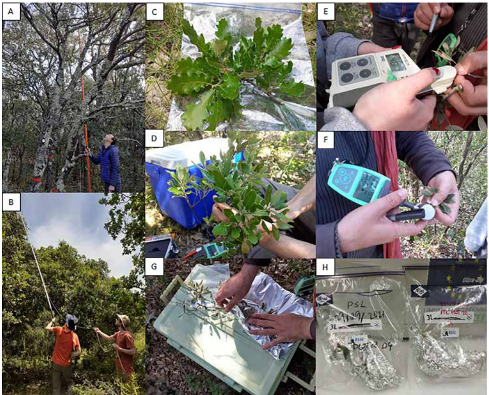
Fig. 18. Photos A and B illustrate leaf sampling at PUE and PSL respectively; photos C and D represent the sampled twigs for QP and QI respectively; photos E and F illustrate measurements with the SPAD and DUALEX respectively; photos G and H illustrate leaf conditioning (photos by Karine Adeline, ONERA).
