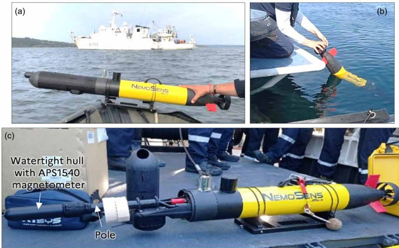
FIGURE 3 NemoSens micro-autonomous underwater vehicle (AUV) (RTSys). (a) AUV ready to dive in front of BH2 Laplace vessel. (b) Launch from the rear platform deck of the hydrographic launch. (c) Watertight hull encapsulating the Applied Physics Systems 1540 vector fluxgate magnetometer tied to the AUV by a pole.
