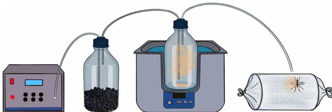
Fig 1. Schematic set-up of the behavioral assay (a: Stimulus controller; b: Gas washing bottle containing activated charcoal; c: Water bath; d: Sample bottle for insecticide or control solution; e: PTFE tubing; f: Cage containing one mosquito female).
