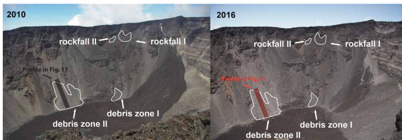
Figure 6. Mapped areas with visible surface changes within the different time steps between 2010 and 2016 that lie inside the derivable DTM. Both highlighted profile lines (grey, red) for the years 2010 and 2016 are analyzed in Figure 11.
