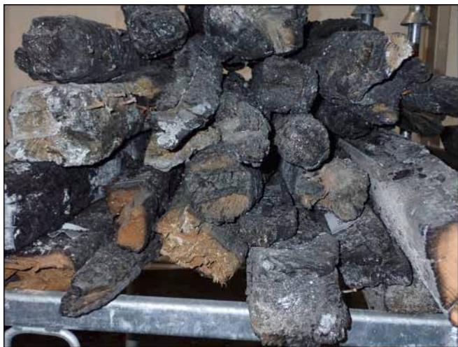
Fig. 1. Example of the carbonisation heterogeneity in the wood beams recovered from the Notre-Dame de Paris cathedral.
