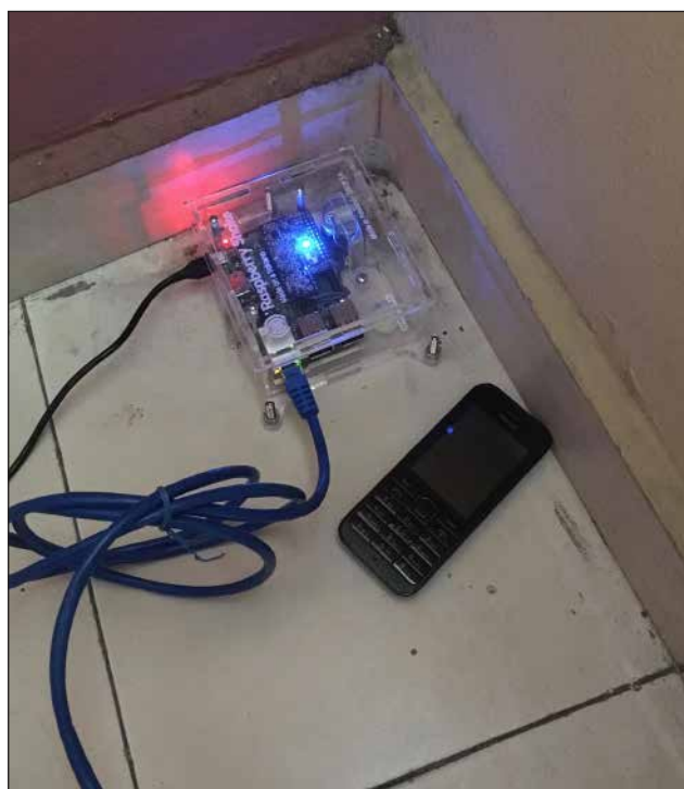
Figure 2 Photo of a Raspberry Shake (RS) seismometer installed at a host located in Port-au-Prince. The RS is lying on the floor in a corner of their living room, behind a piece of furniture that hosts a TV and various electronics. The mobile phone gives the scale. The connection to the electricity (black cable) and the internet router (blue cable) can be seen.
