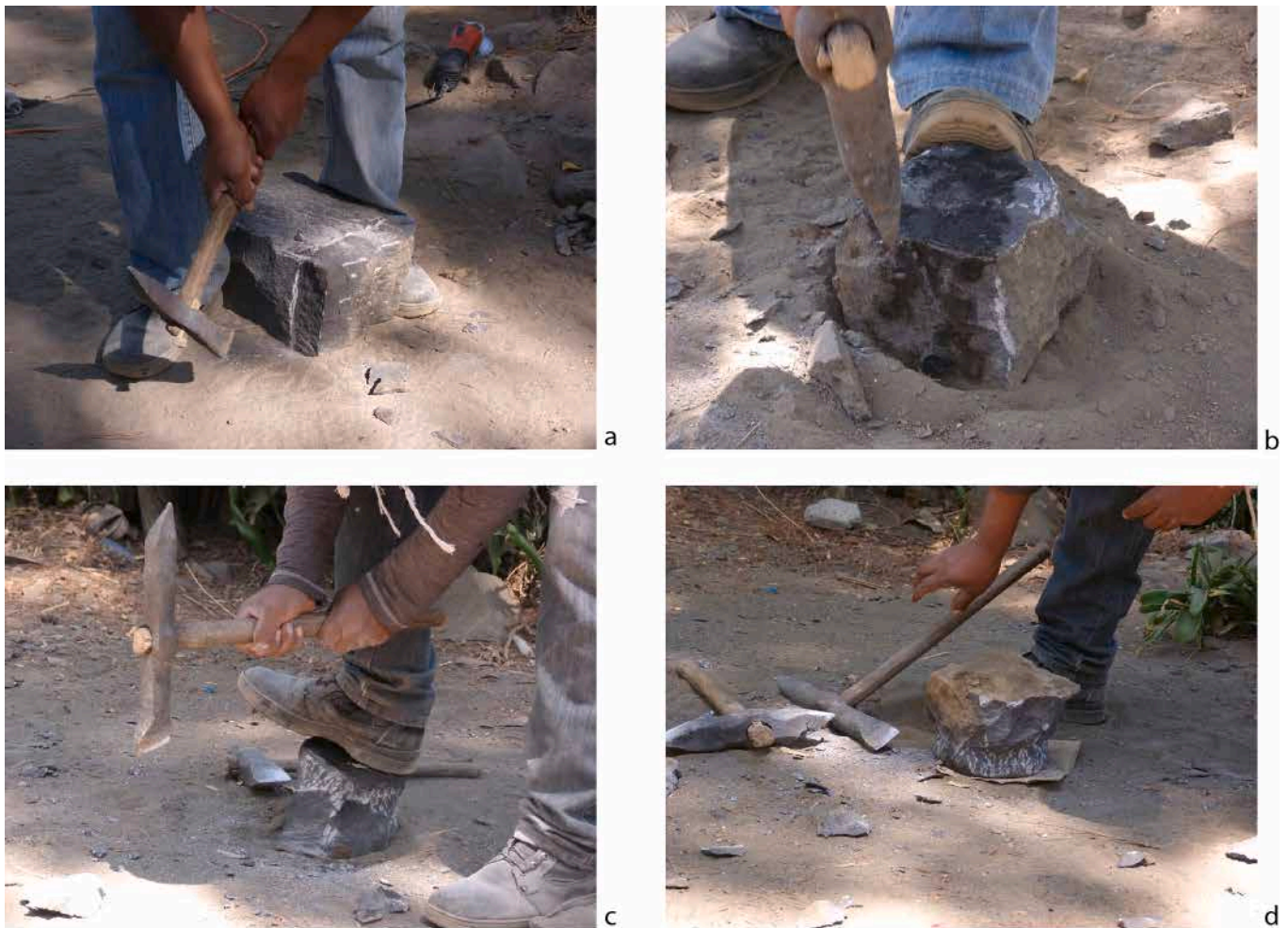
Fig. 13. Molcajete roughing. a) block down-sizing; b) roughout shaping; c) and d) design of the general shape, from bottom to top (photos C. Hamon).
