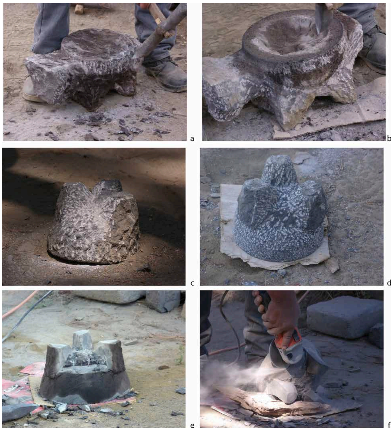
Fig. 15. Shaping the molcajete's sides and feet. a) and b) regularization of the upper side of the bowl; c) and d) shaping and regularization of the feet and downside; e) and f) shaping and regularization of the feet and downside with the portable electric cutting-stone device (photos C. Hamon).
