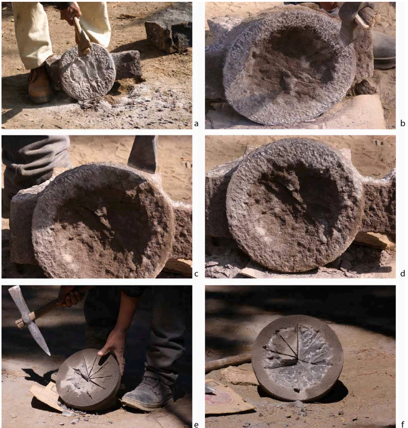
Fig. 14. Hollowing out the molcajete bowl. a) hollowing out inside the round frame with the heavy pick; b) delineating the bowl; c) and d) regularizing and flattening the round frame; e) deep star-shaped incisions at the center of the bowl made with the electric cutting-stone device; f) removal of material with the pick to shape the concavity of the bowl (photos C. Hamon).
