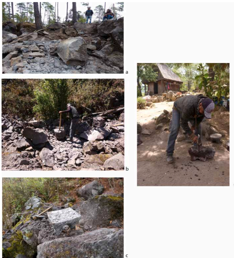
Fig. 4. Workshops (a, c) in the quarry at El Metate volcano with selected blocks surrounding a platform covered with waste. Block extracted (a), to be worked (b) and raw preform ready for transportation (c). Nicolás Vidales working in his parents' domestic workshop (d). In the background is a traditional Purépecha wooden house («troje») that serves as a kitchen area (photos C. Hamon and C. Siebe).
