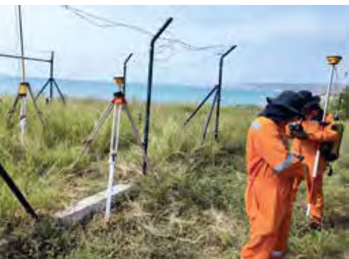
Satellite stations to monitor the coastline and calculate tsunami propagation, Ecuador.
