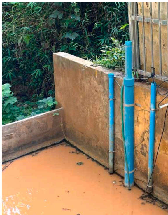
Fig. 27. Field deployment of the self-contained water level gauge at the M-TROPICS critical zone observatory during the 2024 monsoon.
