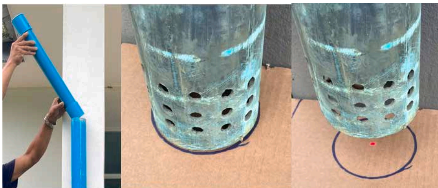
Fig. 18. Checking alignment of the distance meter laser beam. a. Insert the gauge unit at the top end of float guide tube #22; b. Draw a circle of the same diameter as that of tube #22 on a sheet of cardboard; c. Gently move the cardboard sheet away from the end of the tube to check that the beam is as close as possible to the centre of the circle.
