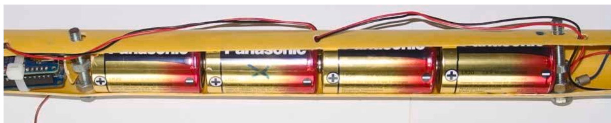
Fig. 10. View showing the installation of the batteries in the electronic module holder #15 and the detail of electrical contacting using bolts and nuts.
