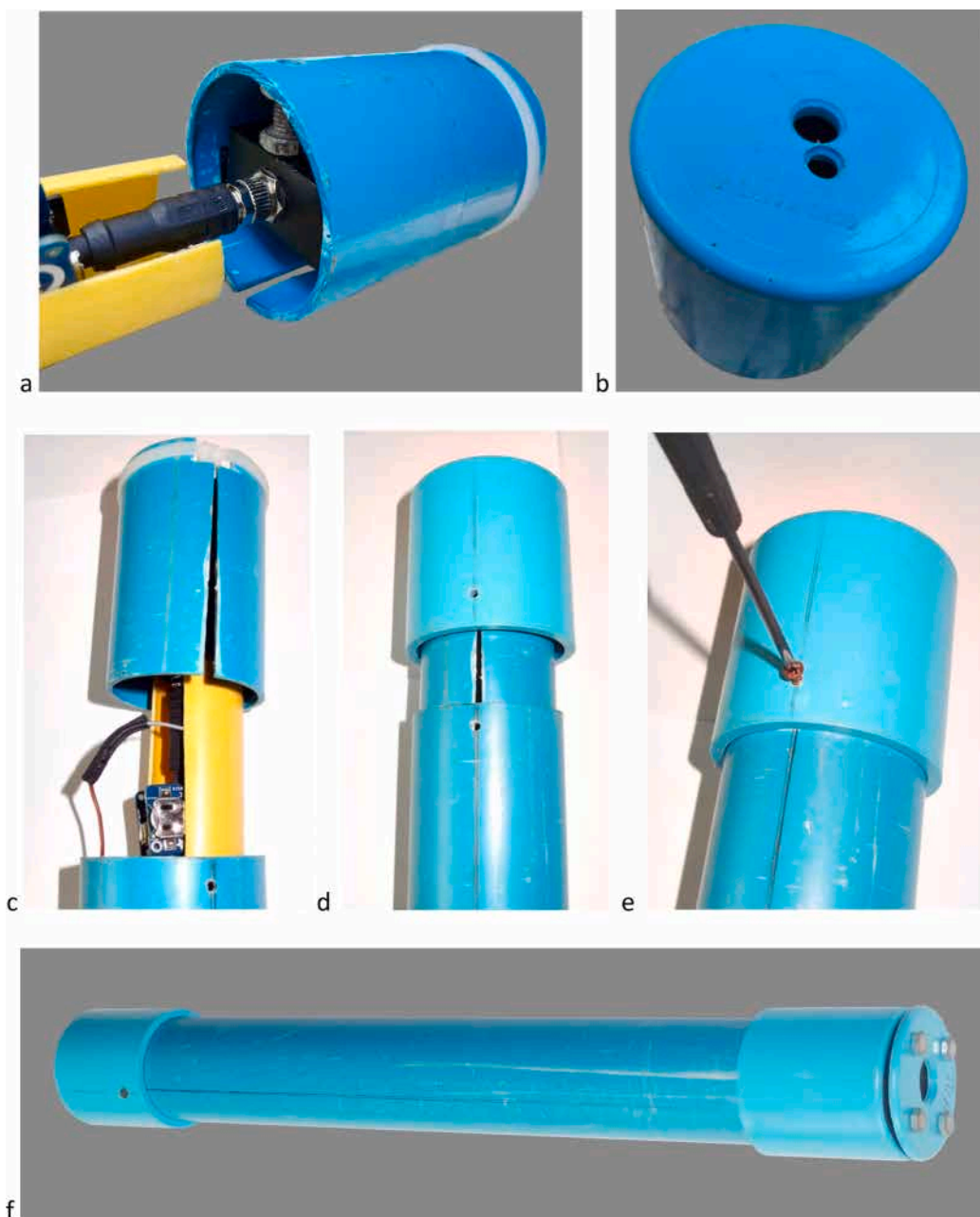
Fig. 13. Final assembly of the gauge unit. a. Close-up showing the end of the electronic module holder #15 (left), the distance meter connector with the metal collar screwed tight (center) and the distance meter unit holder #9 (right); b. External view of the distance meter module cap #1 showing the holes to be aligned with the distance meter emitter and sensor windows when attaching #1 to the external enclosure #10; c. Insertion of the electronic module holder #15 into the external enclosure #10, ensuring slot in the distance meter unit holder #9 is aligned with the hole drilled on external enclosure #10 to receive the locking screw #3; d. Insertion of the distance meter module cap #1 onto the external enclosure #10; e. Final locking of the distance meter unit using the locking screw #3; f. Overall view of the complete gauge unit with distance meter module cap #1 to the left and reset push-button insulating cover to the right.
