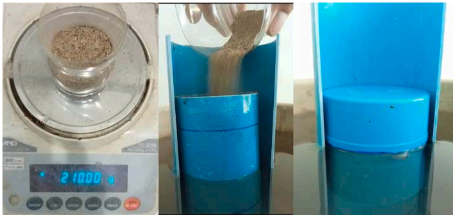
Fig. 17. Preparing the float; a. Weigh the estimated necessary mass of sand; b. Pour sand into the container formed by the PVC tube #19 and sealed end cap #18 until the desired floating line is reached; c. Seal top end cap #20 to finalize the float.
