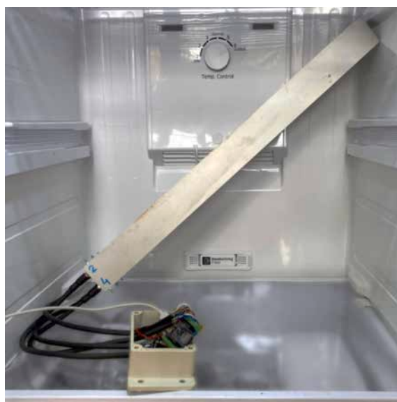
Fig. 23. Picture showing the enclosure containing the four tested units while being submitted to 0–5 °C temperatures in a fridge.
