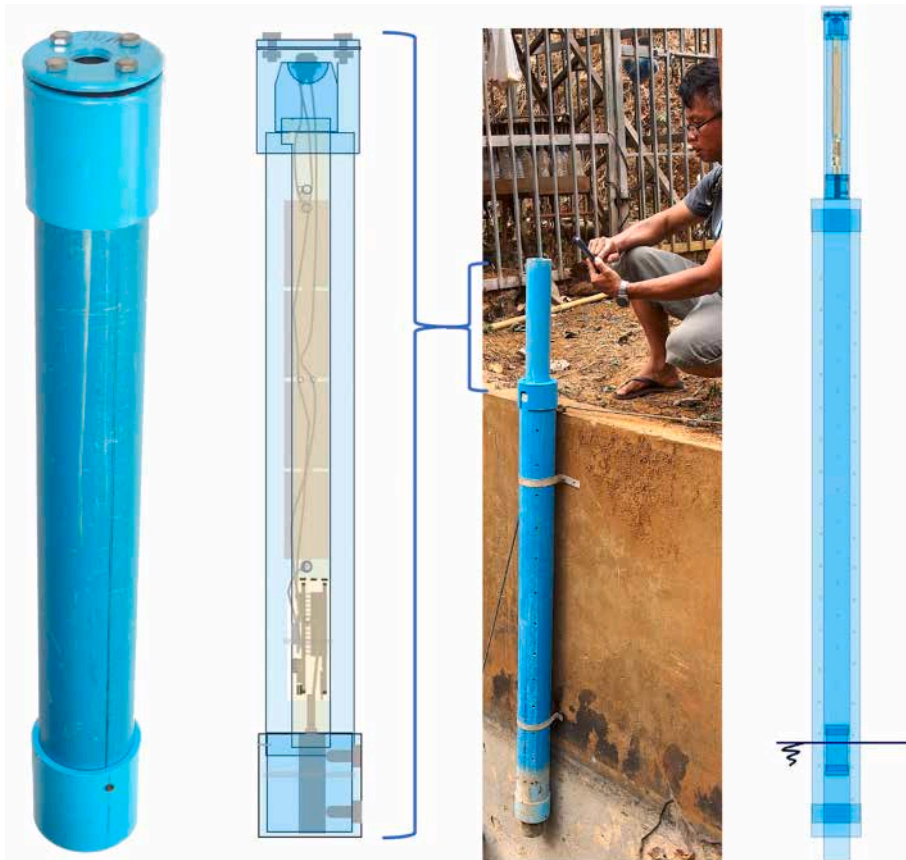
Fig. 2. Overall view of the float-controlled self-contained water level gauge for the monitoring of stream levels. Far left: view of the complete gauge main housing with access to reset switch at the top. Left: transparent view of the gauge's mechanical and electronic components. Right: field setup for water level monitoring in a weir showing the strainer tube fixed to the wall of the weir and the long float guide tube at the top of which the gauge main housing is inserted. Far right: transparent view of the mechanical and electronic components of the field installation.
