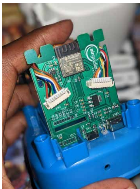
FIG. 4.5B Openaq printed control board (Collins Gameli Hodoli)
