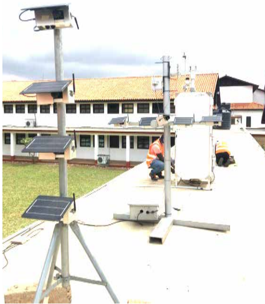
FIG. 4.4A Collocation at UG of LCS (located in the two posts in front of the picture) with fixed reference-grade monitors, which are located inside the white shelter at the back of the picture (Jessica Pourraz)
