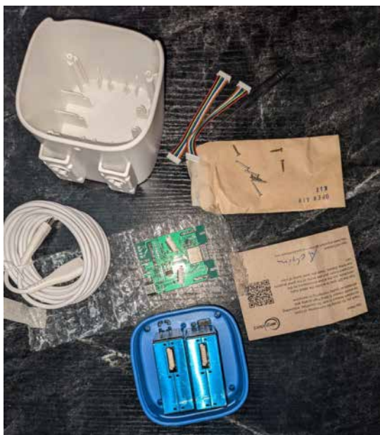
FIG. 4.5A Openaq low-cost sensor kit (Collins Gameli Hodoli)
