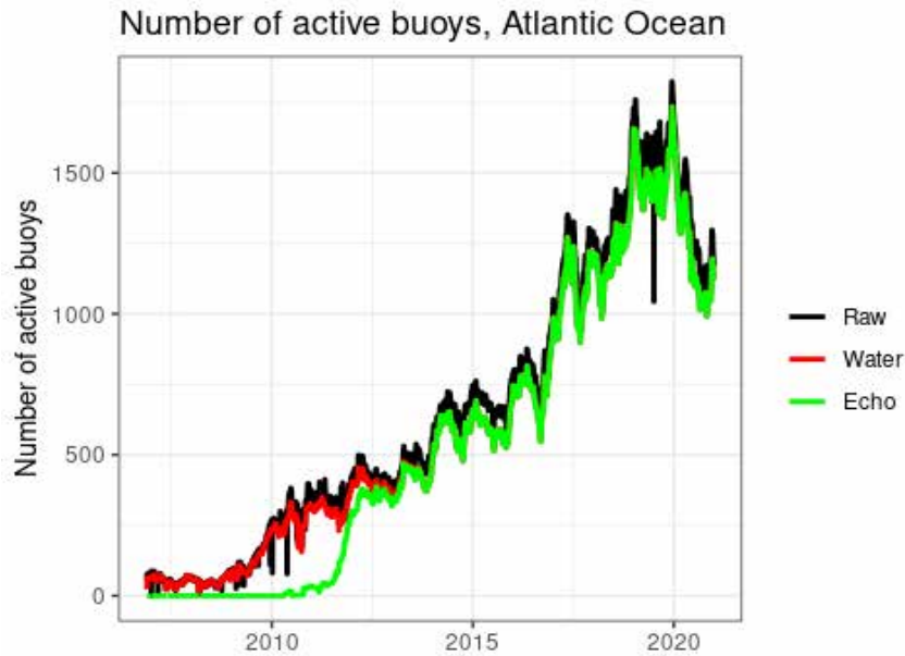
Figure 14. Number of buoys in DB per day, Atlantic. Time series of the number of active (i.e., transmitting position information) buoys per day in the French dFAD tracking buoy database for the Atlantic Ocean. Raw indicates the number found in the raw data including all positions, even those classified as on board a vessel. Water indicates the number of active buoys after filtering out positions that are considered to be on board or beached and after having interpolated over small gaps of at most 4 days (so this amount can occasionally be greater than Raw if missing days are filled in). Echo indicates the subset of Water buoys possessing an echosounder. Note that these estimates do not account for missing data. In particular, the decline in the number of active buoys since 2019 is partially or entirely compensated by missing Satlink trajectory data not found in our database.
