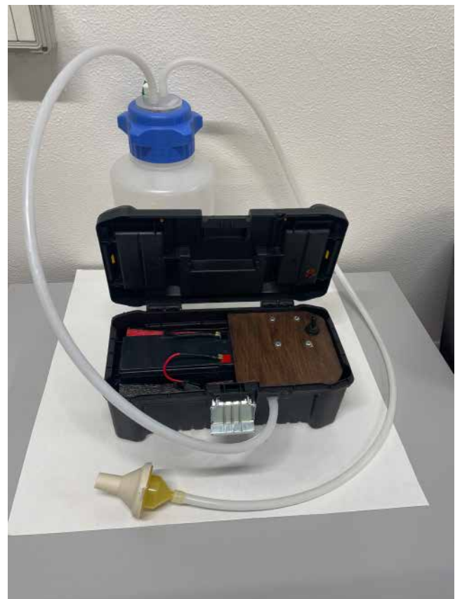
FIGURE 2 | Home-made portable filtration device connected via tubing to a vacuum trap and a filter holder (Smith-Root).
