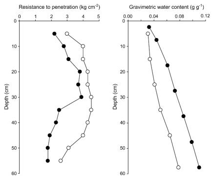
Figure 1. Resistance to penetration measured in the field with a pocket penetrometer. Both wet (-•-) and dry (-o-) conditions are presented with respective gravimetric water content profiles (average and standard deviation associated).
