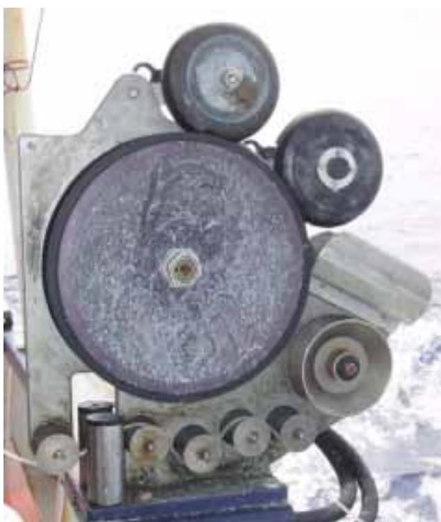
B – The shooter installed astern of the fishing vessel
