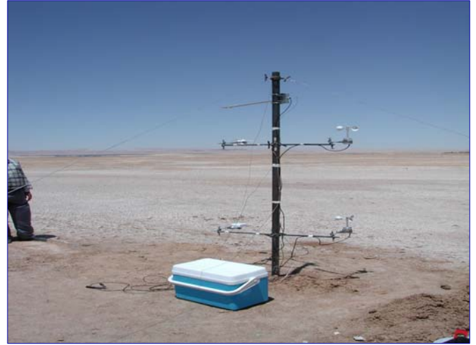
Figure 1 – equipment used in the evaporation measurement from Sabkht Al Mouh
