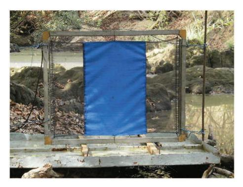
Figure 1. Example of a target design used for comparison. A 0.75 m wide×0.50 m high net-blue-net target (37.5 cm×50 cm blue surrounded by 2 pieces of net of 18.75 cm×50 cm each) inside an electric grid mounted on a fly collection tray. doi:10.1371/journal.pntd.0001332.g001
