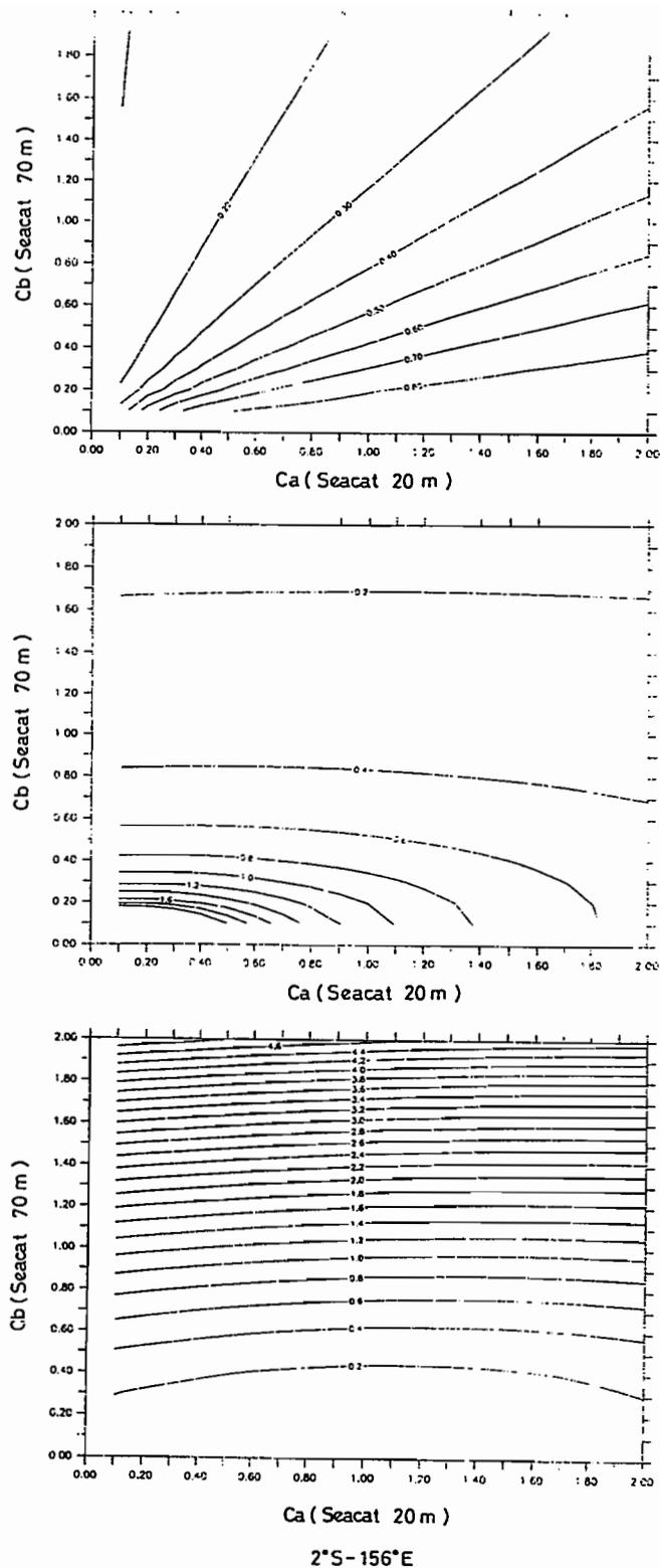
Figure 4. Determination of the Ca and Cb coefficients. For the Seacat with incomplete temperature at 30 m: (a) correlation between the measured and interpolated series (COR), (b) ratio of standard deviation of measured series versus standard deviation of the interpolated series, (c) rms difference between the measured and interpolated series.
