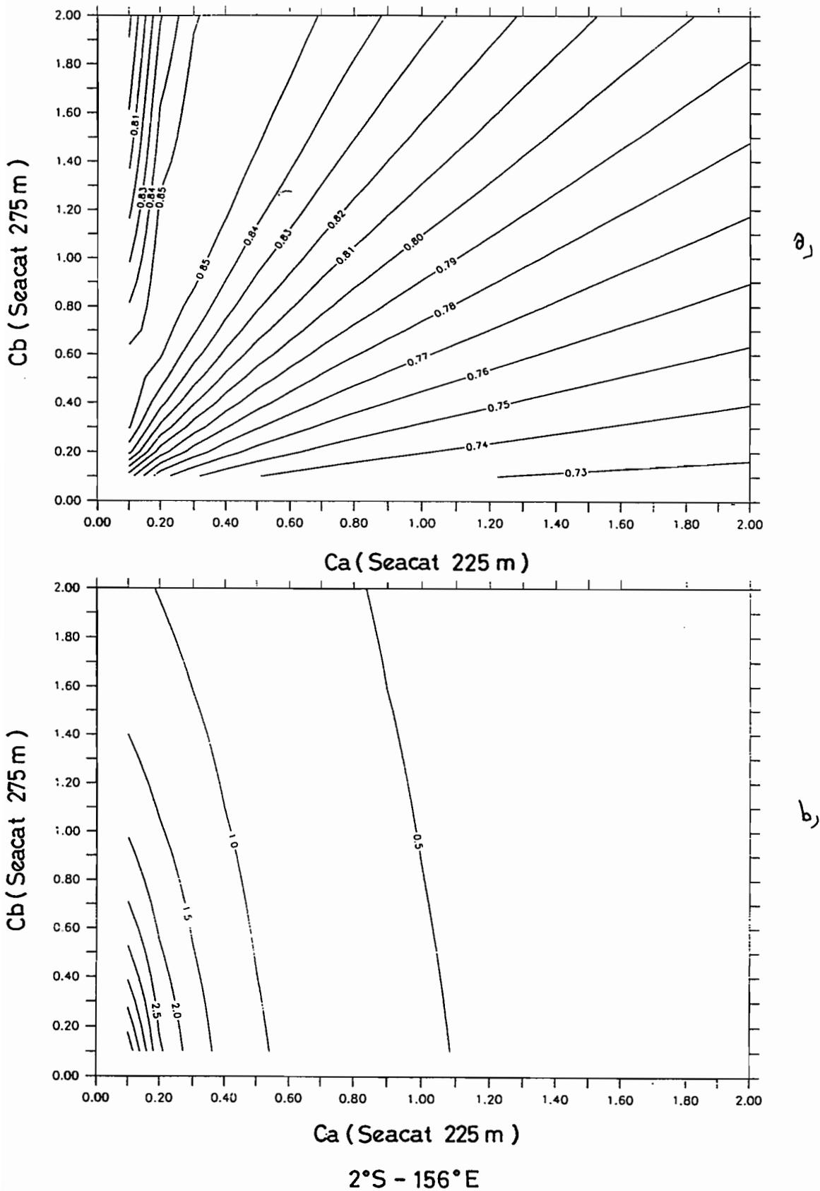
Figure 7. Determination of Ca, Cb coefficients used to interpolate the daily ATLAS temperature at 250m ( $2^{\circ}\text{S}$ - $156^{\circ}\text{E}$ ) at a 5-min rate using the 5-min Seacat information at 225 m and 275 m adjacent to the ATLAS sensor. (a) Correlation between the measured and reconstituted ATLAS series (COR), (b) ratio of standard deviation of measured series versus standard deviation of the interpolated series for the daily ATLAS.
