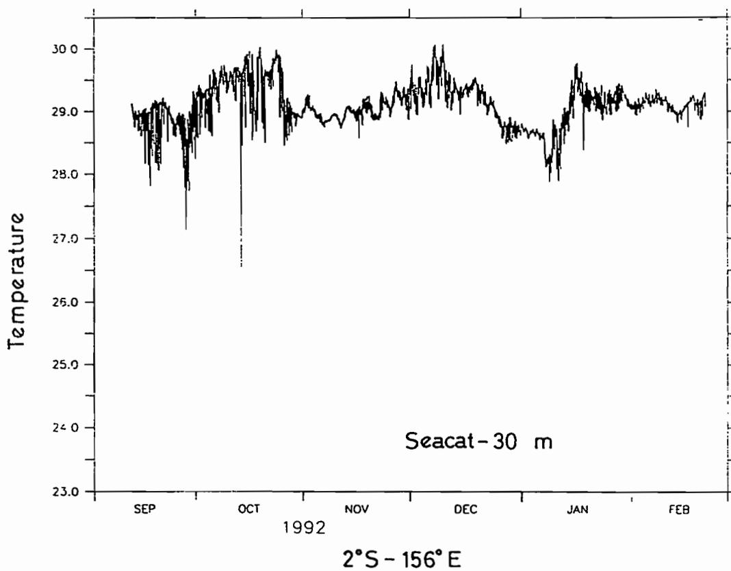
Figure 5. Final 5 min Seacat temperature series at 30 m interpolated using Ca, Cb coefficients of 1.1 and 0.1 respectively.
