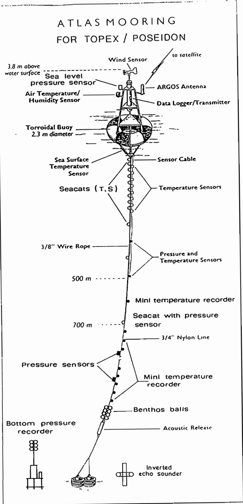
Figure 2. ATLAS mooring design with additional instrument along the line (Seacats, Mini Temperature Recorders, benthos balls), and on the bottom Inverted Echo Sounder and Bottom Pressure Recorder.
