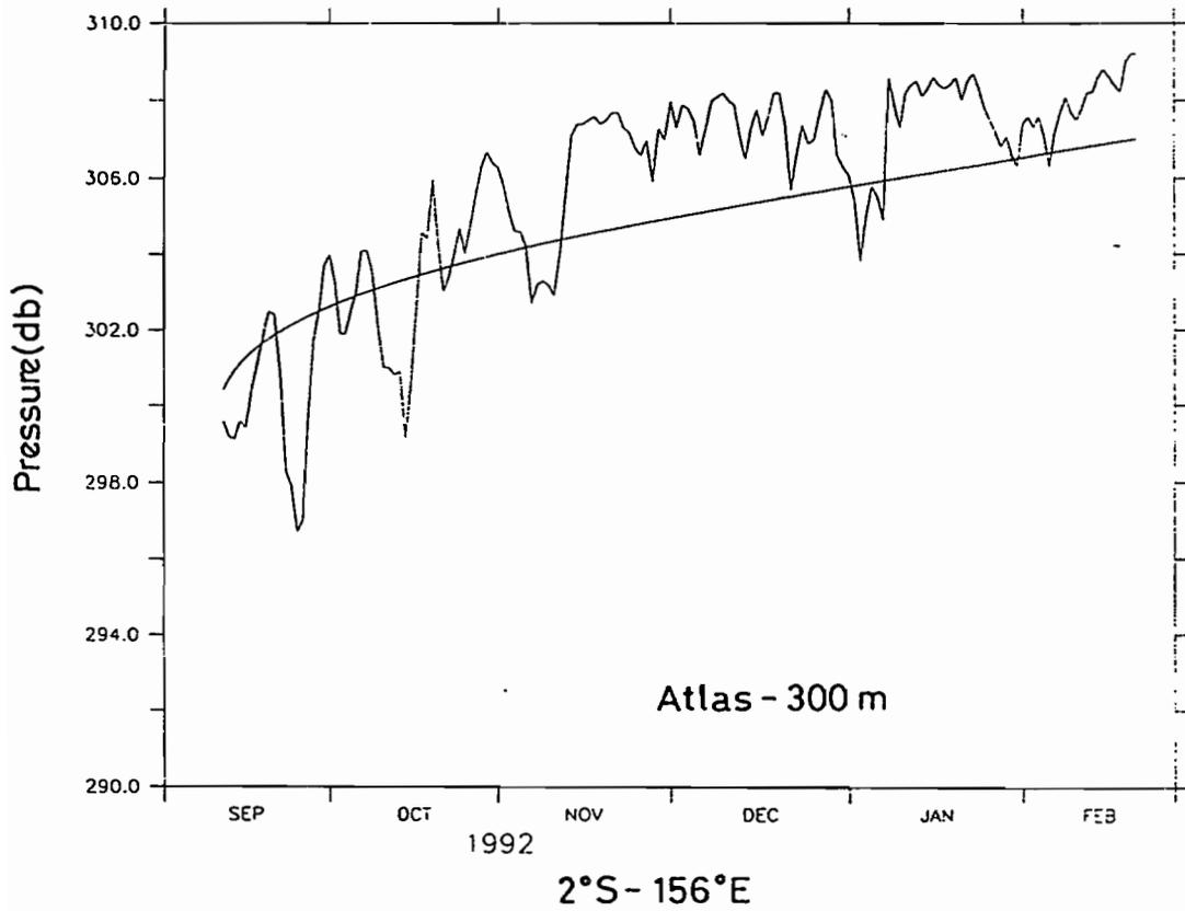
Figure 8. Evidence of the drift in the original daily ATLAS pressure (dbar) at 300 m (2°S-156°E). The drift is fitted by a function F defined in the text.
