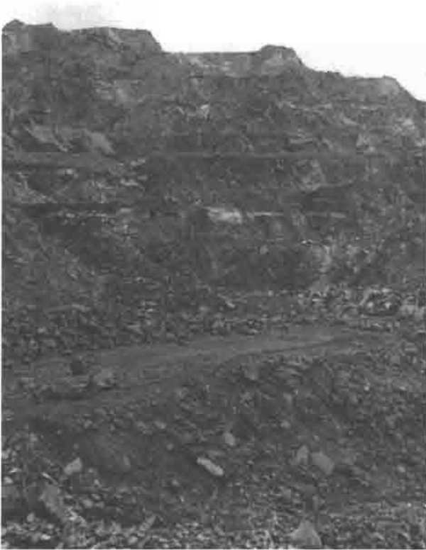
PLATE 4. Quarrying for Nickel Ore on the Thio Plateau, Showing Terraced Forms Produced by Excavation at Successively Lower Levels
