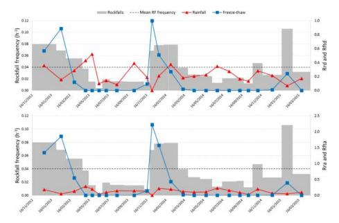
Figure 7. Rockfall frequency for the different observation periods, with rainfall and freeze—thaw duration ratios (up) or rainfall and freeze—thaw amount ratios (down).
