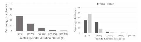
**Figure 4.** Distribution of rainfall episodes duration, and of freezing and thawing periods duration. More than 80% of thawing episodes are shorter than 12h, and almost 95% of thawing periods are shorter than 24h. Long thawing periods occurred only at the end of the winter, when freezing no longer occurs.
