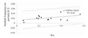
**Figure 8.** Simple linear regression between rainfall amount ratio (Rra) and rockfall frequency for dating periods without freeze—thaw. Dashed grey lines: 95 % interval confidence.
