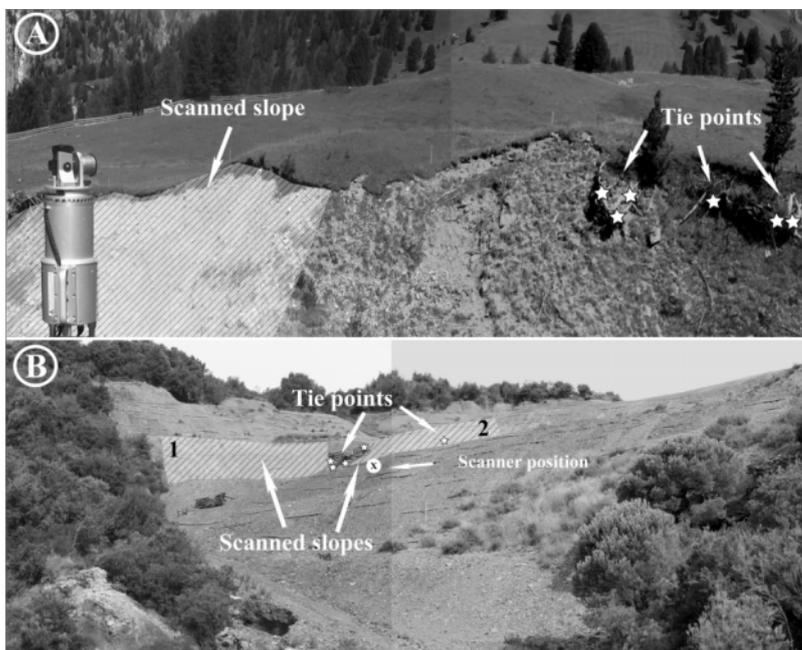
**Fig. 2** Scanned slopes in the Val di Funes valley (A) and on the slopes at Rio Marina/Elba (B) and the locations of the fixed tie points.
