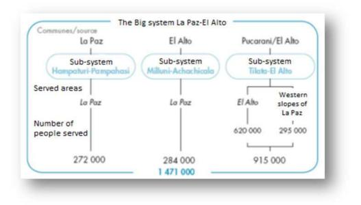
Figure 1 - The "Big" water system in La Paz-El Alto
