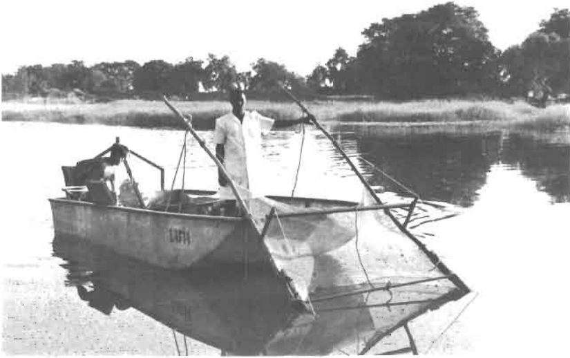
Photo 14 An electrified front trawl, experimented in Lake Chad.
