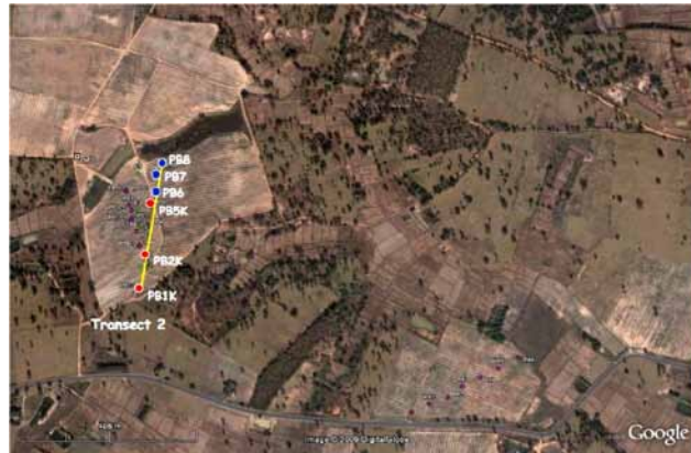
Figure 2. Location transect piezometric along the southern slope of the watershed. In red, the deepest piezometers (length exceeding 25 m); in blue, the shallower piezometers (length of about 12 m)
