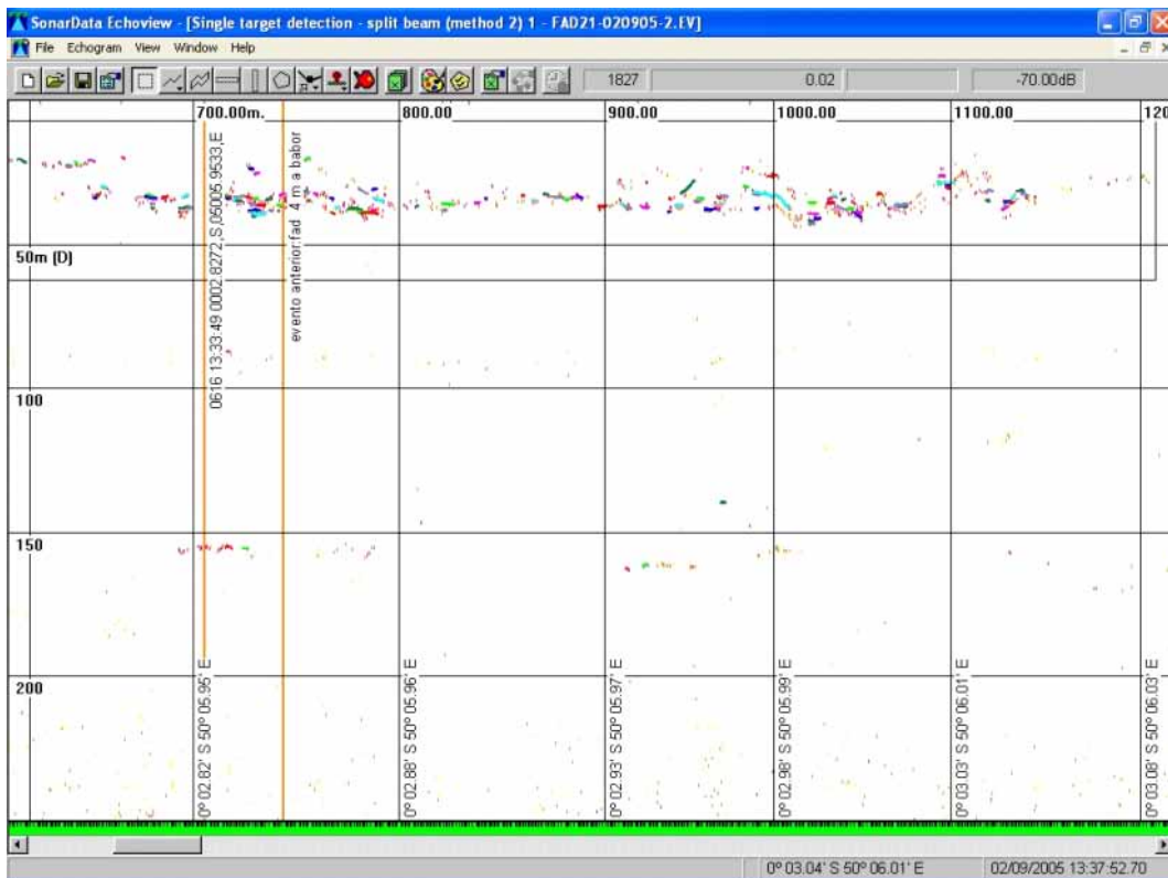
Figure 15. Example of an echogram showing a group of tuna located under an object following the vessel for approximately 500 m.
