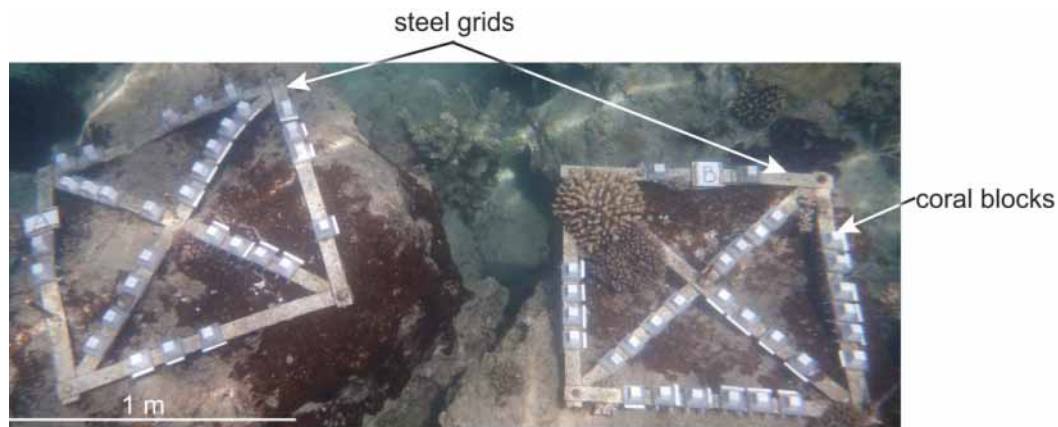
Figure 44 Two of the four grids installed on the study site at the 'Ile aux Canards' in New Caledonia. Thirty coral blocks per grid were fixed and exposed between 1 and 12 months to the colonization by microborers.
