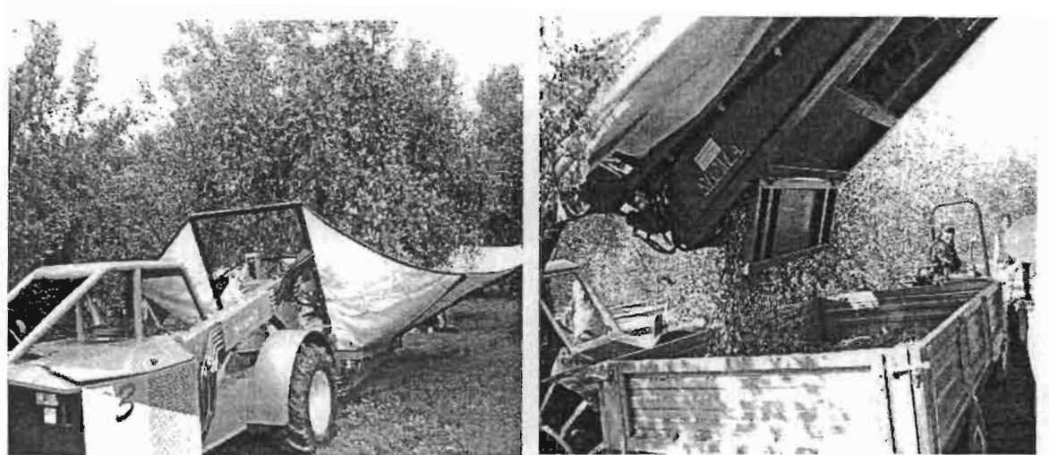
Photo 1: The olive mechanical harvesting by trunk shakers with reversed umbrella interceptor.
