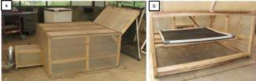
Figure 6-3 Hand-made oven used in Depok; a) overview; b) inside view
