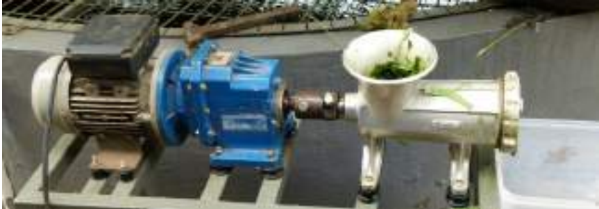
Figure 7-2 Small chopper used to crush plants into growth substrate for BSF larvae
