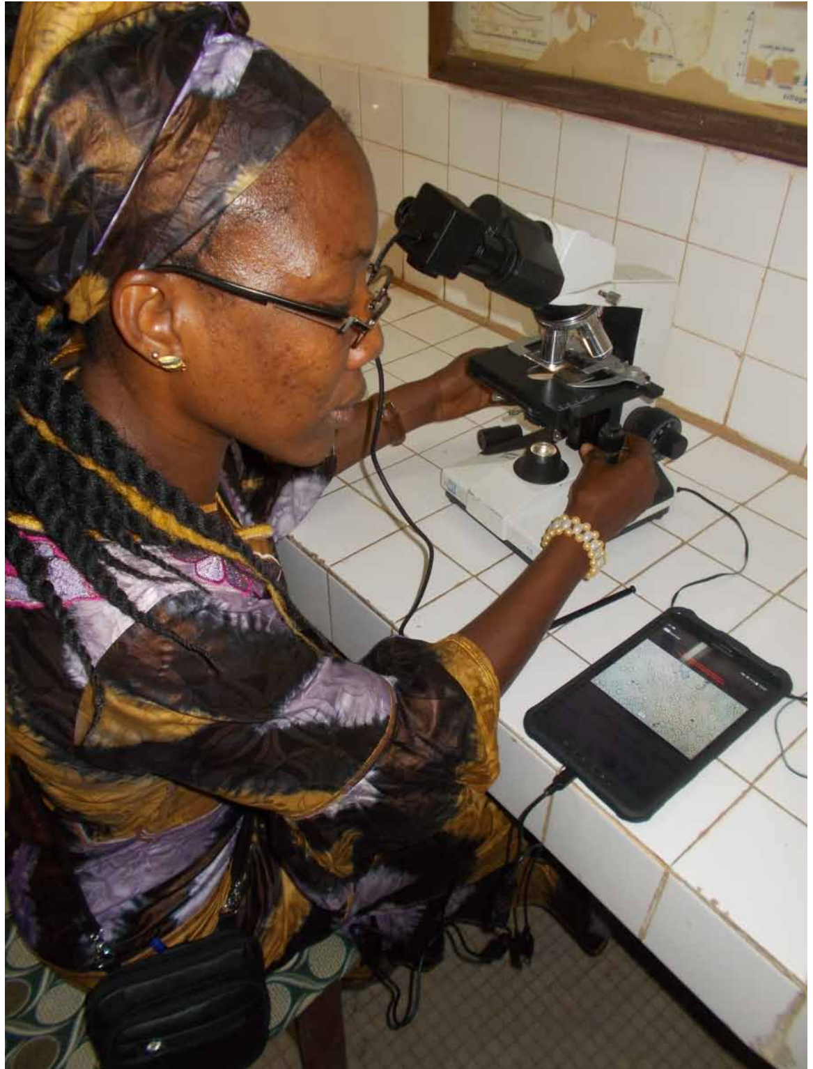
Fig 2. Digital imaging system for recording videos of microscopic images using an android tablet and external camera mounted onto the ocular tube of a microscope.
