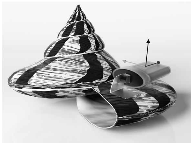
Fig. 2 Large Trochus ( B_d = 120 mm) instrumented with accelerometer. HOB0 Pendant G data logger was attached to an aluminum tag. The arrows indicate the three measurement axes of the accelerometer
