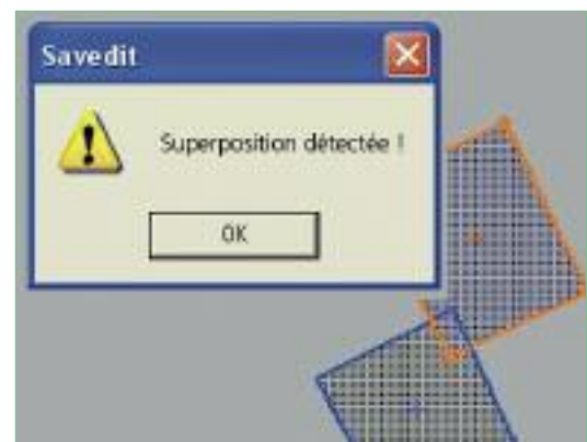
Third type of error capture: partial overlap of two zones that creates a third
