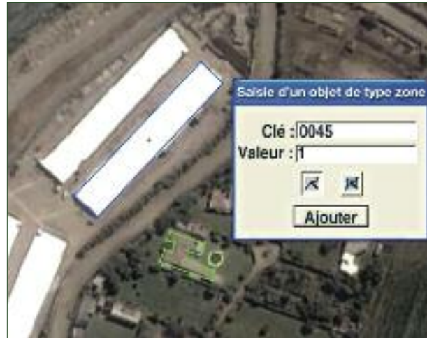
Display of an image and outlining of the buildings in a GIS publishing module
