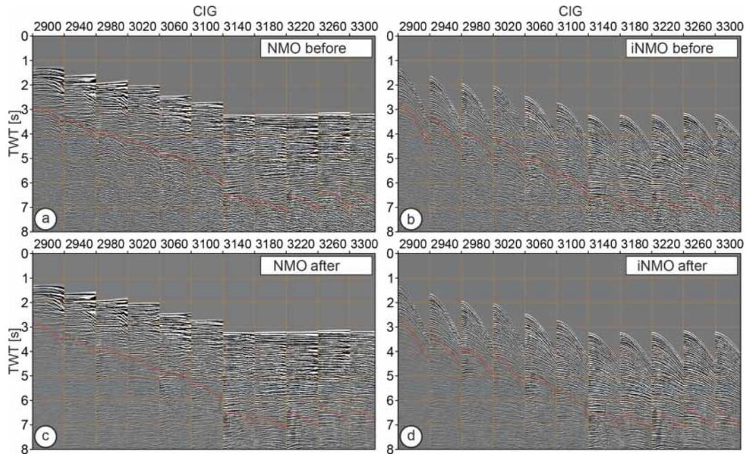
**Figure 4.** CIGs converted to time domain (a–b) before and (c–d) after radon multiple attenuation. Gathers in (a)–(c) are NMO-corrected, while gathers in (b)–(d) have inverse NMO applied. Red dashed curves delineate the estimated position of the multiples.
