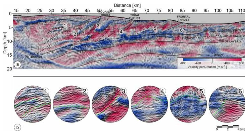
**Figure 12.** Imaging results and structural interpretation. (a) Migrated section superimposed on a de-trended version of the FWI velocity model, blended with the average vertical and horizontal velocity gradient. (b) Zoom panels corresponding to circles 1–6 in Fig. 12a. Green dashed lines underline the consistency between reflectivity and background velocity perturbations.
