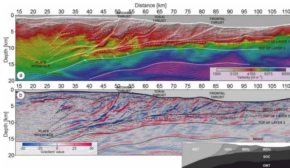
**Figure 11.** Imaging results and structural interpretation. Migrated section superimposed on the following: (a) the FWI velocity model blended with the average vertical and horizontal velocity gradient; and (b) the average vertical and horizontal velocity gradient of the FWI model. Inset presents different geological block segments: OMT – oceanic mantle; SOC – subducting oceanic crust; WDU – weakly deformed unit; MDU – moderately deformed unit; HDU – heavily deformed unit; BST – backstop.
