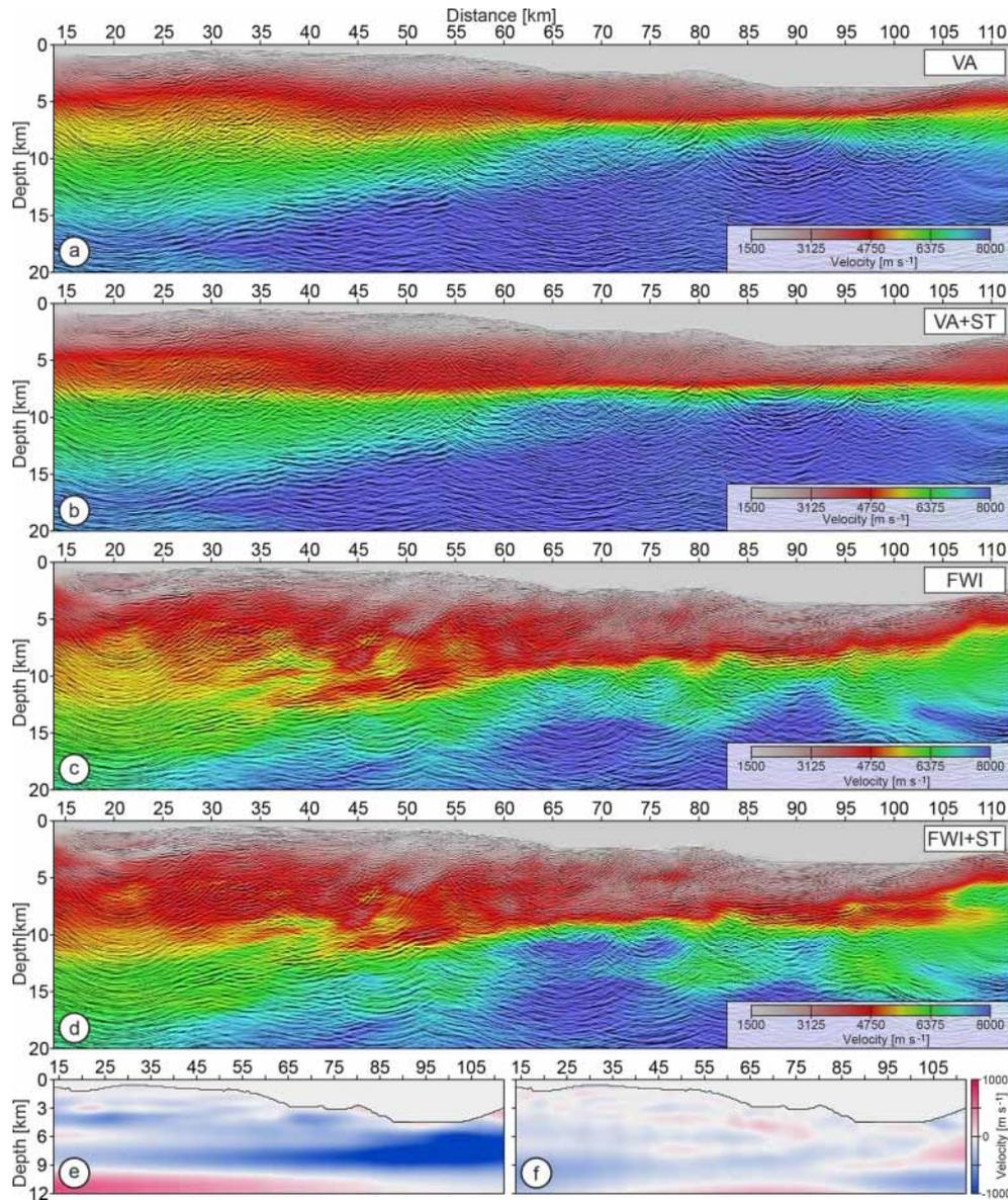
**Figure 8.** PSDM sections inferred from the (a) VA, (b) VA+ST, (c) FWI and (d) FWI+ST velocity models displayed in the background. Velocity perturbations introduced by ST into the (e) VA and (f) FWI velocity models.
