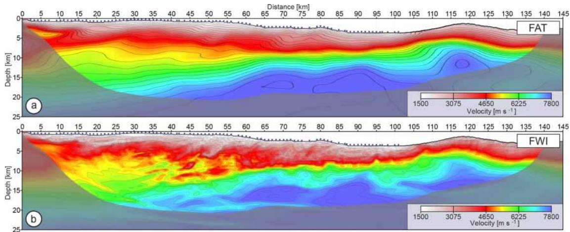
**Figure 3.** Velocity models derived from the OBS data using FAT (a) and FWI (b). Triangles at the seafloor represent positions of the OBSs. Note that there is no OBS coverage above 102 km of distance. Shading mask corresponds to the area not covered by first-arrival rays.
