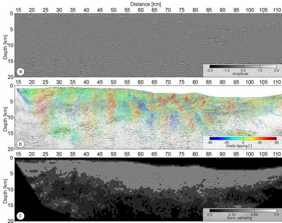
**Figure 7.** (a) PSDM section inferred from the FWI velocity model. (b) Cloud of the scattering points corresponding to picked slopes. Colors represent estimated dipping of the interfaces. (c) Normalized average sampling of the model space by the scattering points superimposed over the PSDM section from (a).
