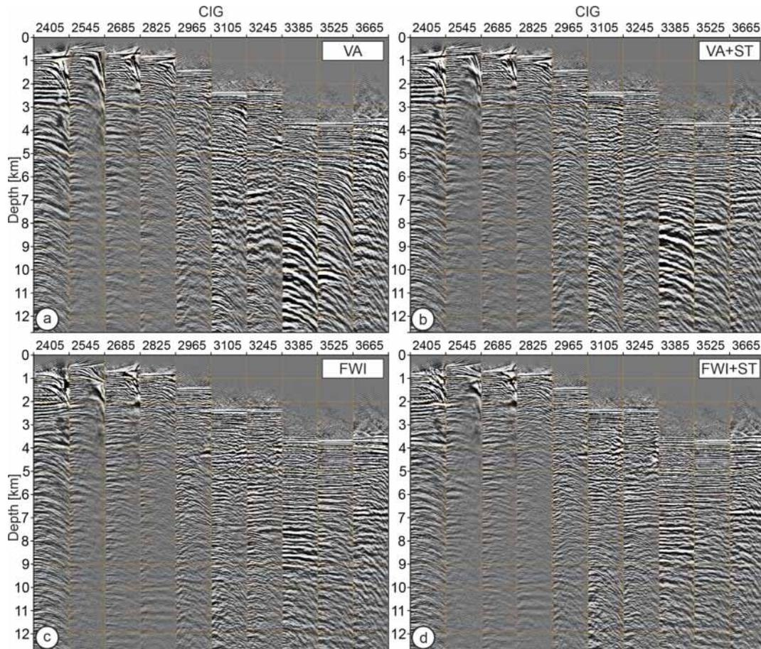
**Figure 9.** CIGs extracted along the whole profile (every 8.75 km). (a–b) CIGs inferred from the velocity model built by (a) VA and (b) VA+ST. (c–d) CIGs inferred from the (c) FWI and (d) FWI+ST velocity models.
