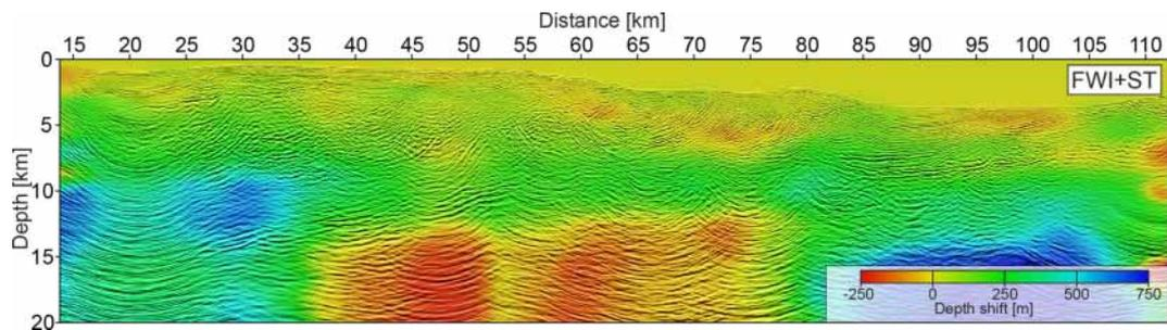
**Figure 10.** PSDM section inferred from the FWI+ST velocity model overlaid on the estimated depth shifts. Positive and negative values correspond to upshifts and downshifts introduced in the PSDM section by FWI+ST velocities relative to the FWI velocities, respectively. Note the nonsymmetric color scale.
