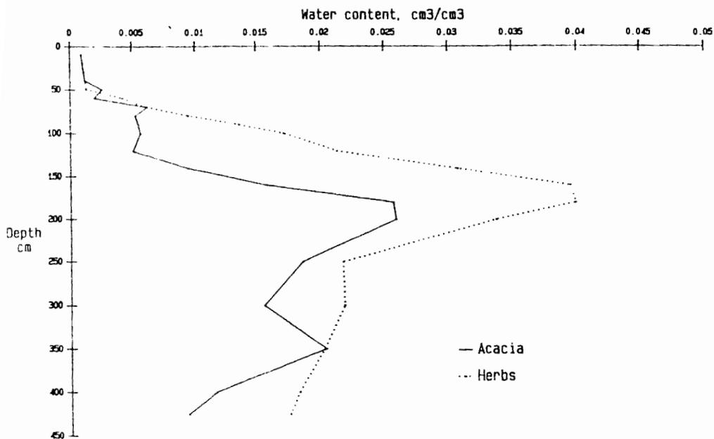
Fig. 4b. Soil-water content profiles
