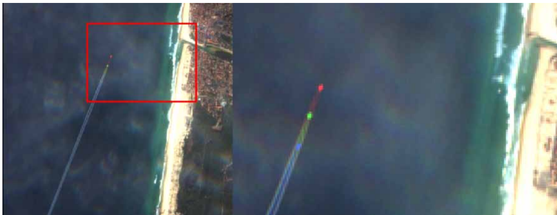
Figure 1. Illustration of the time-lag between detector bands B02 (blue), B03 (green) and B04 (red) by the different colors of the flying airplane at Capbreton, France. The time-lag between each band is 0.527 s.
