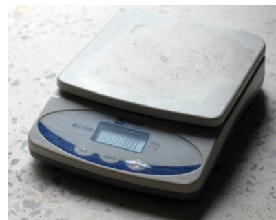
Figure 32: Balance used for small animals (0.1 g precision) (Photo: Herbreteau V.)
