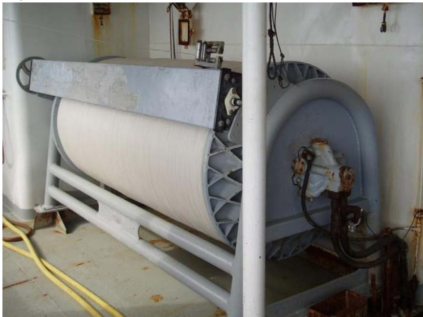
A - The spool by Lindgren Pitman™ installed on board the longliner
