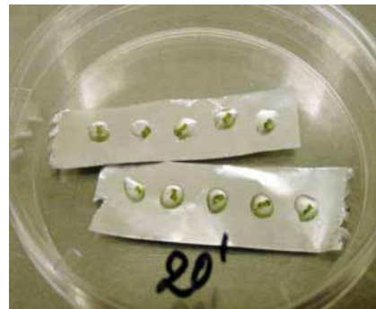
Fig. 2. Foil strips with explants in droplets of vitrification solution - Rubus fruticosus , droplet-vitrification
