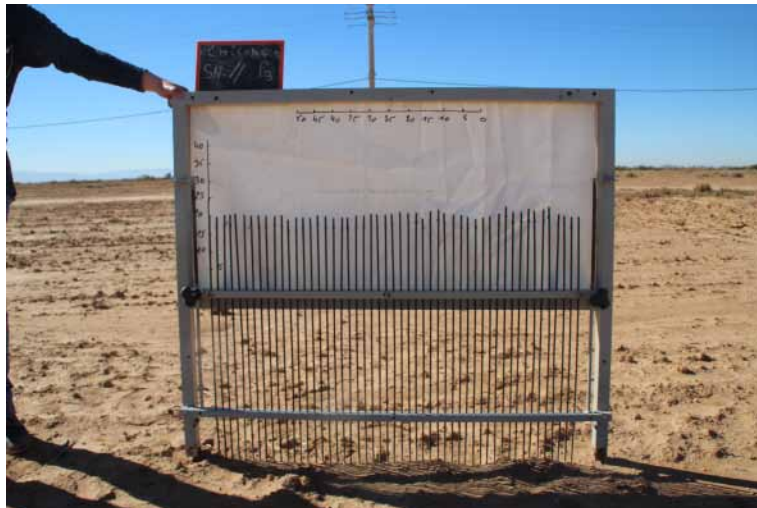
Figure 2. Example of the needle-profilometer used in this study.
