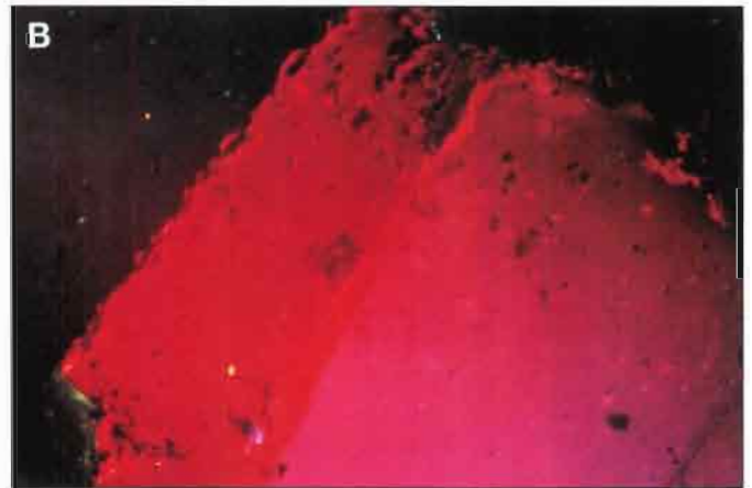
■ Fig. 3. Transmitted light (A) and cold cathodoluminescence (CL) photographs of a Muzo trapiche emerald. Note that the green overgrowth (A) corresponds to the red orange part in the CL image (B), a small more bright border underlines the contact between the rose-red core and the red orange overgrowth zone. Width of the photograph 2 mm.
