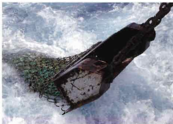
Figure 485: The sturdy Warén Dredge used to sample mixed and hard bottoms.
