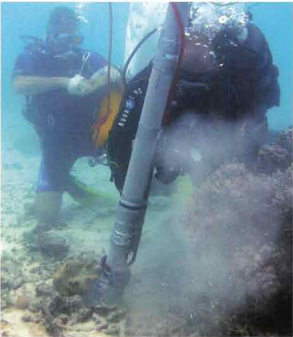
Figure 483: The air-operated suction sampler in operation by SCUBA divers.
