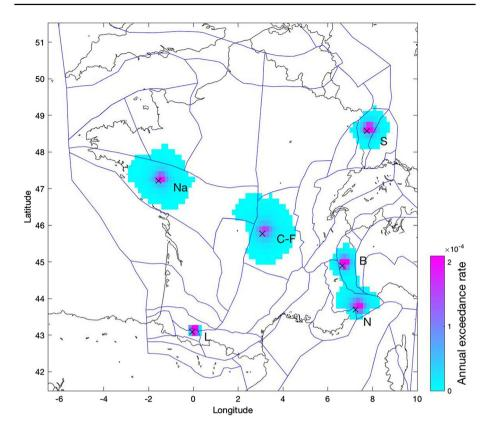
Fig. 10 Spatial disaggregation for the six cities studied for the PGA at 475 year return period. The spatial cells that contribute up to 98% of the total exceedance rate are displayed. The Baize et al. (2013) seismogenic model is combined to FCAT catalog; Bindi et al. (2014) is used to predict ground-motion exceedances. Na, Nantes; L, Lourdes; C-F, Clermont-Ferrand; S, Strasbourg; B, Briançon; N, Nice
