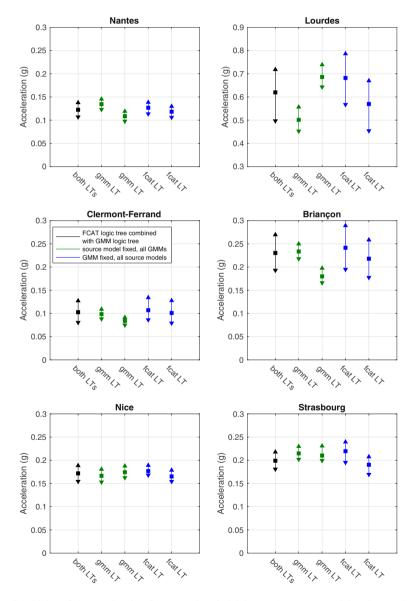
Fig. 15 Sensitivity of the acceleration for spectral period 0.2 s to the source model and ground-motion model uncertainties at a 475 year return period. See Fig. 14 legend
