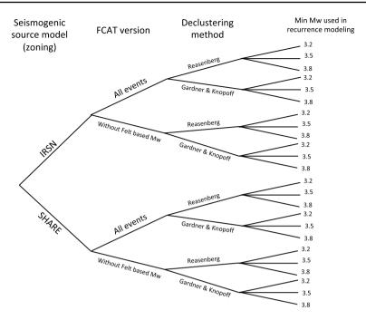
Fig. 11 Logic tree exploring uncertainties on earthquake recurrence models considering FCAT, including two alternative seismogenic source models, two alternative versions for FCAT (all events and without felt-based  $M_W$  events), two alternative declustering algorithms, and three alternative minimum magnitudes
