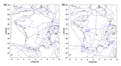
**Fig. 6** Seismogenic source models used in the present study. **a** ESHM13 model (Woessner et al. 2015); **b** IRSN model (aggregated version, see the text for modifications in source zones R-04 and O-02/O-03) (Baize et al. 2013). Probabilistic seismic hazard calculations are performed for the six selected sites (stars) in Sect. 5
