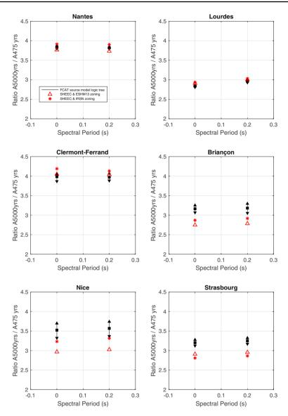
**Fig. 16** Ratios between accelerations at 5000 and 475 year return periods for the PGA (0 s) and the spectral period 0.2 s. Square and triangles: exploration of the FCAT source-model logic tree, mean and 16th and 84th percentiles. Red symbols: ratios estimated from two source models based on SHEEC (triangle: combined with ESHM13 seismogenic source model; star: with IRSN model). Calculations performed with the Boore et al. (2014) ground-motion model
