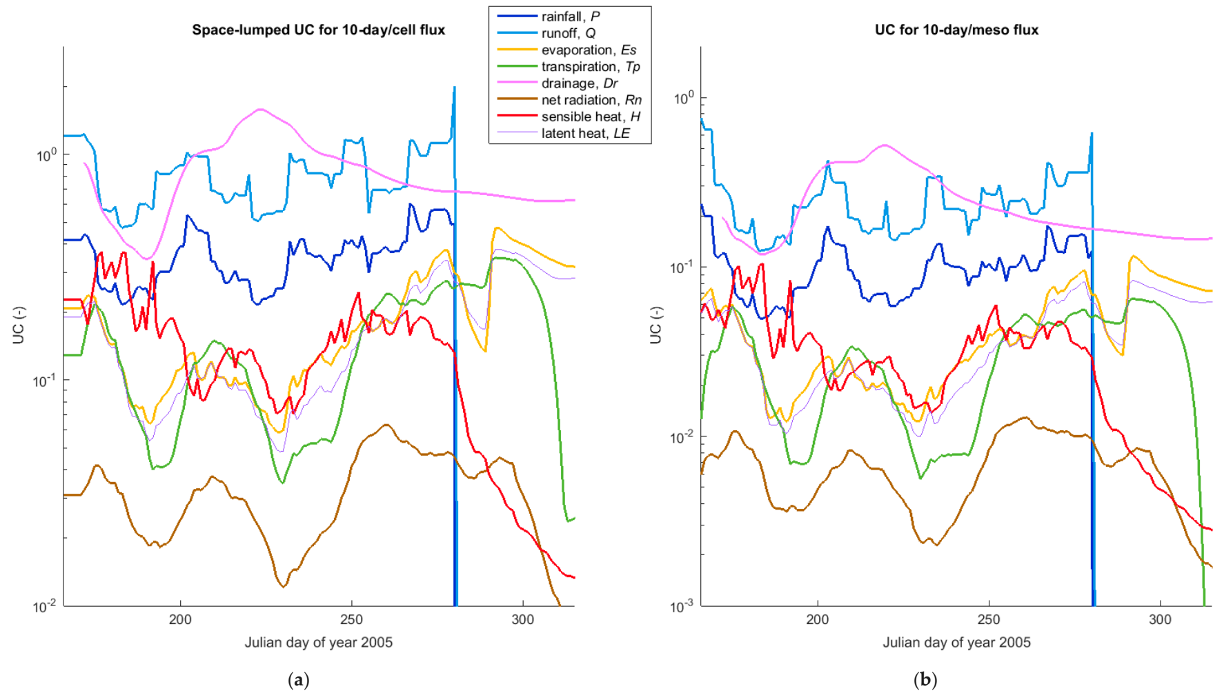
Figure 8. Time course of 10-day scale flux uncertainty coefficients (UC), for (a) cell (with spatial lumping of UC), or (b) meso spatial flux scales.
