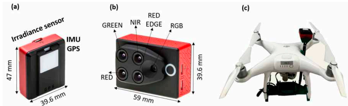
Figure 5. Lightweight unmanned platform highlighting the Sequoia's accessory piece (a), the Sequoia (b), and its package placed in the 3D mount onboard the DJI Phantom 4 UAV (c).
