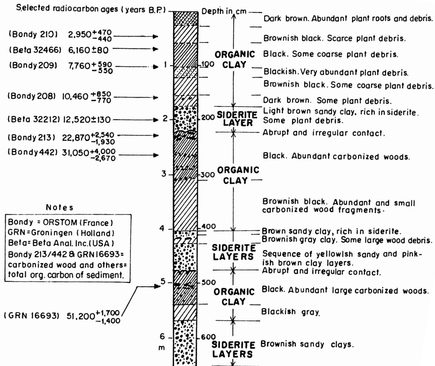
Figure 2 - Lithologic log of the core CSS-2 ("Carajás Serra Sul").
