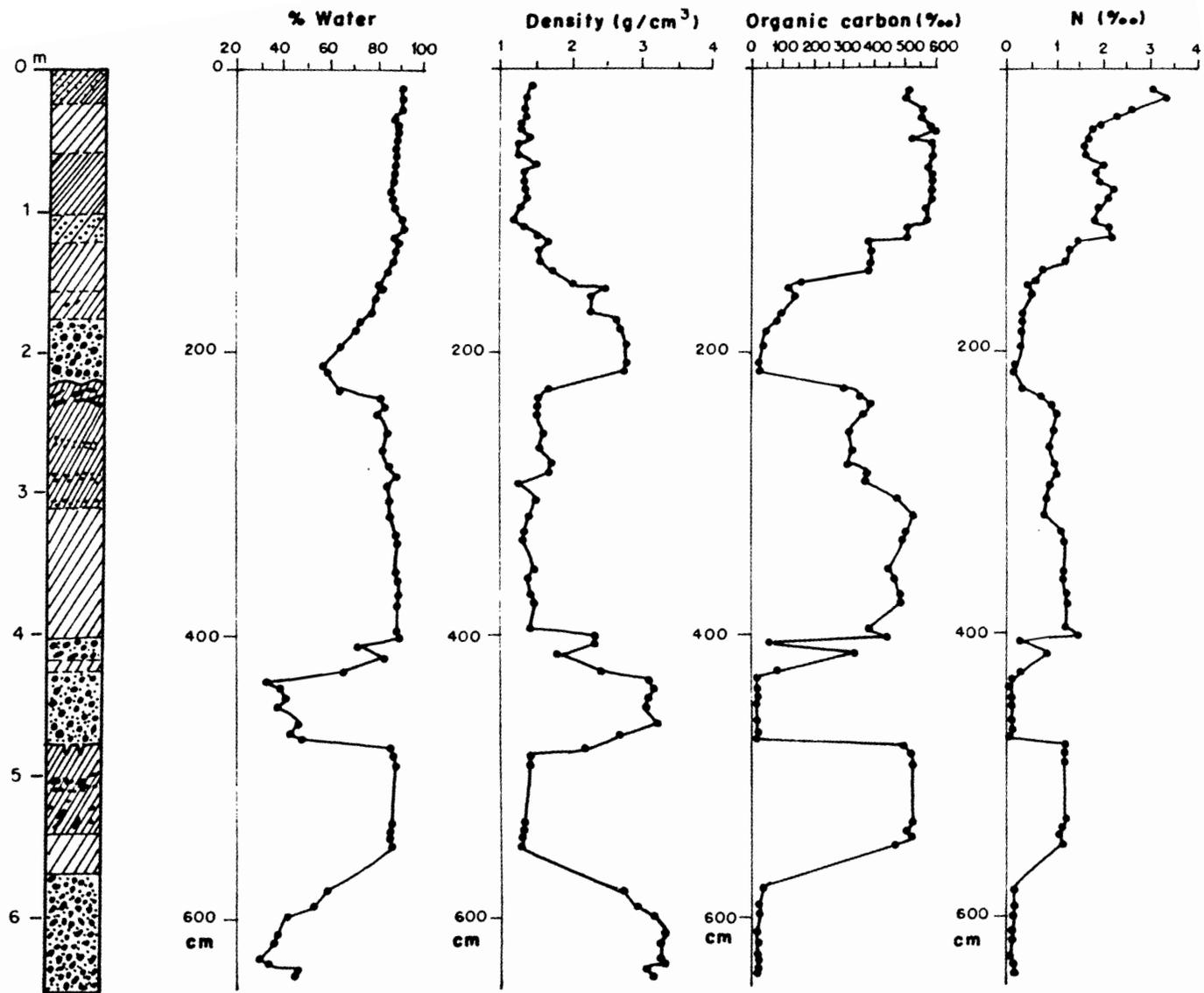
Figure 3 - Densities and water, organic carbon and nitrogen contents of the CSS-2.
