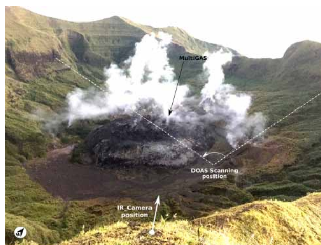
Figure 2. Awu lava dome in the crater. Degassing occurs from the lower crater wall, and the northern part of the crater is the main degassing zone. The positions of DOAS scanning, MultiGAS (MG), and infrared camera are highlighted. The arrow of the IR_cam denotes the direction of the thermal camera.
