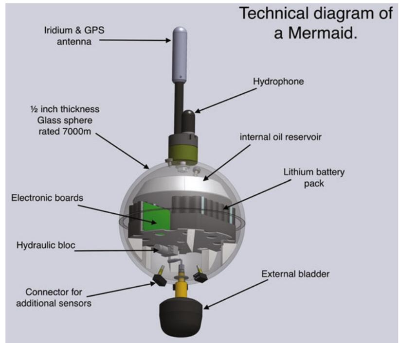
calculates its speed and activates the pump or opens the valve to maintain a speed that varies according to the distance to the desired depth. For the ascent, the float will leave its cruising
