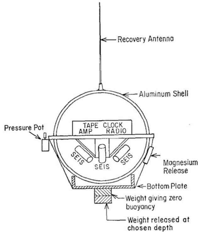
**Floating Seismographs (MERMAIDS), Fig. 1** The spherical float used by Bradner et al. (1970) to record microseismic noise
