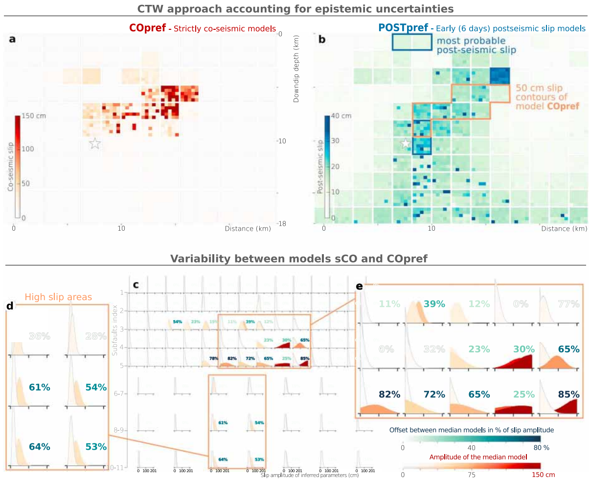
Figure 5. (a) and (b) Strictly coseismic COpref and early postseismic POSTpref (6 days after the mainshock) preferred slip models (norm of the slip vector), inferred with the CTW approach and accounting for epistemic uncertainties. (c) Comparison between the posterior probability density functions of the dip-slip parameters of models COpref (a) and sCO (Figure 3c), colored from the amplitude of their median model. In the last four rows, the PDFs have been merged, covering two subfaults along strike and two subfaults along dip (i.e., patches 2 times bigger than for the first four rows). The COpref model PDFs are in the foreground, while the sCO PDFs are in the background. The offset between the median models is shown as percentage with a different color scale. Two high slip areas are illustrated in detail: the highest slip patch (e) and the deep slip patch (d). The plots of the posterior PDFs are truncated between 0 and 200 cm to simplify the visualization. CTW = Combined Time Windows.
