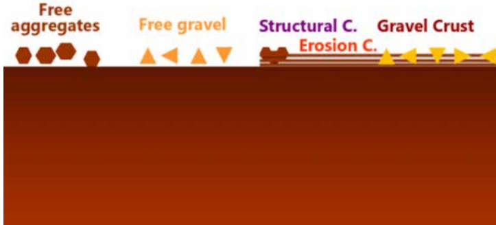
Figure 2.1. Free aggregates and coarse elements, structural crust (embedded aggregates), erosion crust and gravel crust (embedded coarse fragments). For a color version of this figure, see www.iste.co.uk/valentin/soils5.zip
