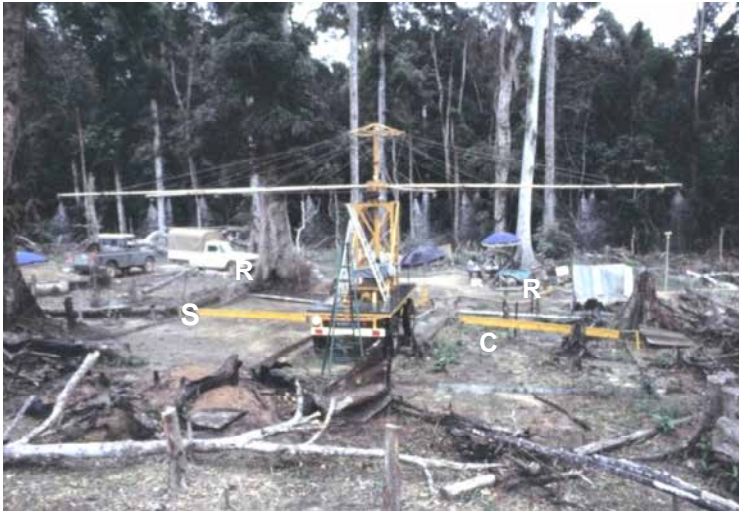
Figure 3.8. Swanson-type rotating rain simulator, watering 200 m 2 in which two runoff and erosion plots 10 m long and 5 m wide are installed, making it possible to compare two treatments, here: bare soil tilled in the direction of the slope (standard treatment, S) and a field prepared for rain-fed rice after slashing and burning (C). Two linear rain gauges (R), in yellow on the photo, make it possible to ensure the homogeneity of the rain on the two plots [COL 84], Taï forest, Ivory Coast (photo: C. Valentin). For a color version of this figure, see www.iste.co.uk/valentin/soils5.zip .
