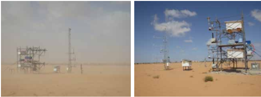
Figure 3.15. Device for measuring vertical fluxes of dust using the gradient method, during a field campaign in southern Tunisia in March–April 2017 (ANR WIND-O-V 4 project). Note that the mast is equipped with cup anemometer profiles, 3D sonic anemometers and thermocouples to measure dynamic parameters, in addition to scaffolding used to collect dust particles according to their size at two levels (left photo) and to continuously measure their concentration by size class and their mass concentration, also at two levels (right photo) (photos: IRD, J.L. Rajot). For a color version of this figure, see www.iste.co.uk/valentin/soils5.zip .
